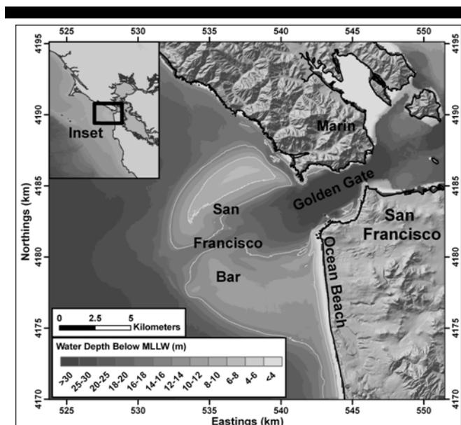
Figure 1. Regional map showing the location of Ocean Beach, the Golden Gate, and the San Francisco Bar. The 10 and 15 m contours are shown in white.
