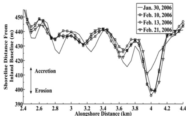
Figure 4. MHW shoreline position relative to a shore parallel inland baseline from four consecutive surveys in the winter of 2005/06. Position is corrected for natural angle of shoreline.
